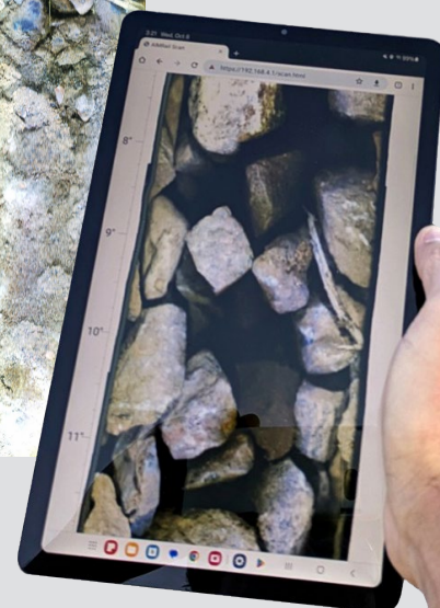
Close up of screen showing the ballast underground
