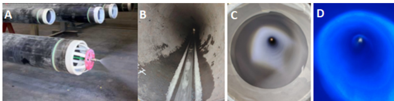
Figure 1: (a) Radial ID Surface Treatment. (b) Pipeline Interior as Received. (c) Pipeline after Preparation/Cleaning (d) Pipeline after treatment under UV illumination.
